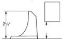
1319FS-3 For door clearance from 1/8" - 1/16" (28.58) - (39.69)mm
